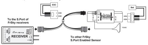
Warning: Install FrSky Smart Port Current Sensor – FAS100S on any appropriate surface of the airframe that stays away from water, vibration, or fuel.
